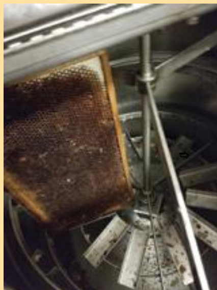
Inside a radial extractor with a brood frame inside for show.
