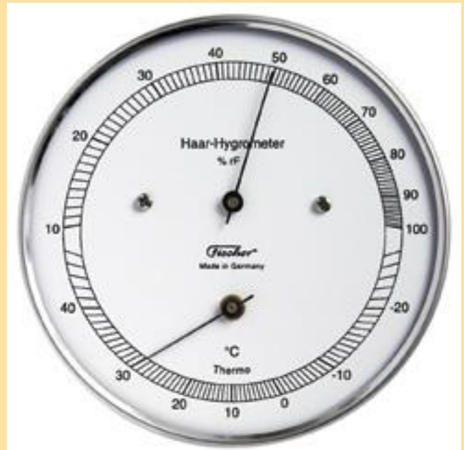
A good hygrometer can be a useful tool in a honey house.
