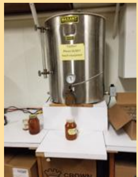
A water jacket bottler. Note the elevated stand to allow easy bottling.
