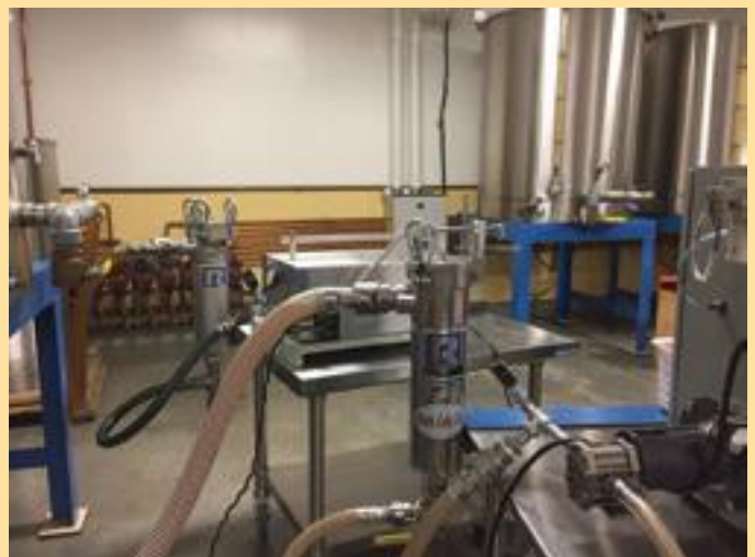
A filter with an 800 to 1000 micron mesh can remove large debris while allowing desirable substances through. ⇨
