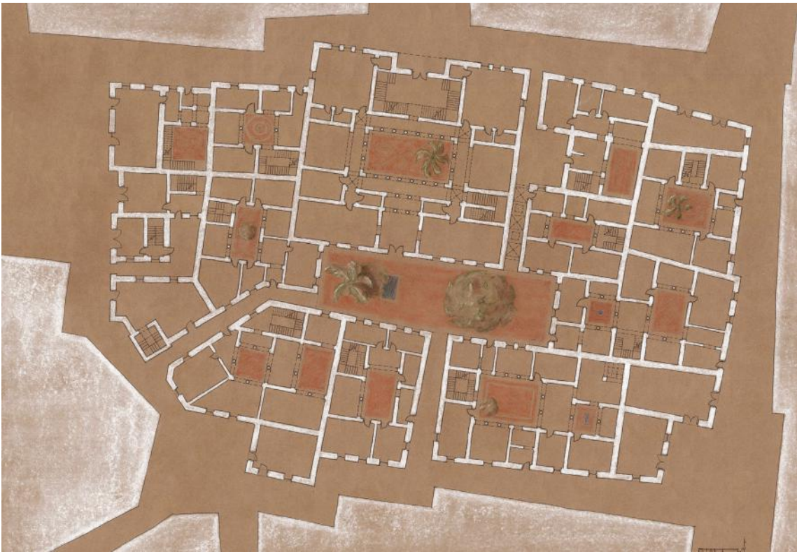
This page: Aerial View and Plan of the typical mixed-use block structure for the reconstruction of Aleppo. This block is composed of a limited number of traditional courtyard houses grouped around a shared half-public courtyard. It offers excellent climate comfort, privacy, and flexibility as a design paradigm. Completed by Cynthia Sigler and Sean Gaoutte for Design VI, Professor Lucien Steil, Spring 2018.
