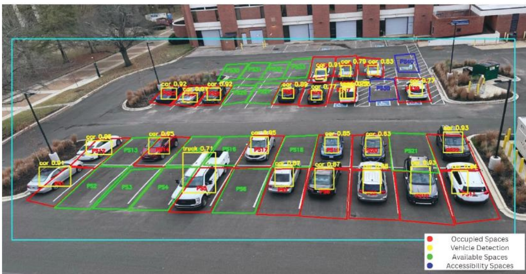
Figure 1. Camera-based parking occupancy detection results for the test lot, showing mapped spaces and detected vehicles used to compute real-time availability.
