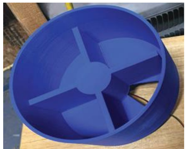
The heart of our Project, the autoloader. The final design will hold 8 payloads of treats and food.
