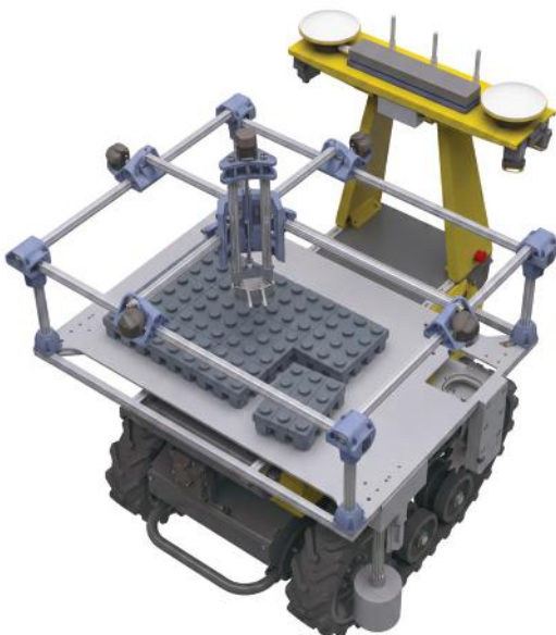
3D model of planting system attached to unmanned ground vehicle (UGV)
