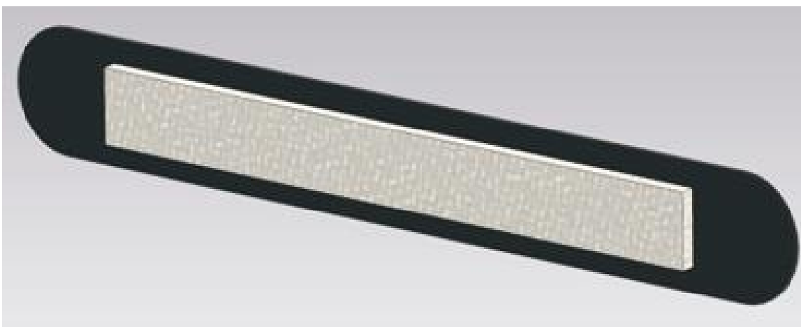
CAD Model of Weighted Tape with Encapsulated Tantalum
