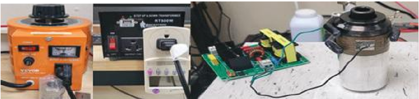
Figure 1: Experimental Setup with Variable Voltage Regulator, Step Up & Down Transformer, and Circuit Board with Transducer Connected (pictured left to right)
