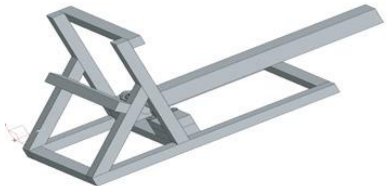
3D CAD design of the automated elephant feeding catapult mechanism
