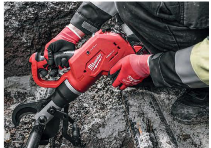
Above: the tool can be lowered into position where the parrot-beak jaws can be easily swung into the target to capture the material and then remotely activated to complete the cut. Spare cutter blades are readily available.
