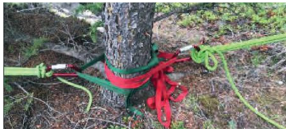
Above: A focused anchor with pre-tensioned back ties and interwoven W3P2 webbing on the tree.
