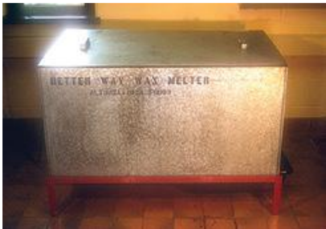
This is a 1986 converted slide photo of a Betterway Wax Melting that was in my lab. It was a very useful device. Under strict supervision, the device could even be misused as a honey liquefier. As I recall, it measures about 30" high x 45" long. It could take maybe 30-40 frames at the time. The edge of catch pan is underneath the melter at the right. The resulting overheated honey was not fit for human consumption. Rendered wax floated on top of the hot honey. Plastic foundation and foundation inserts were destroyed. Rendered frames could be refurbished and were reasonably disease and pathogen-free. The overheated honey still had specialty uses while the resultant wax was re-rendered in smaller batches. This was not a device for processing wax that was still almost white wax. As with solar melters, this machine was too rough on such delicate wax. After my retirement, this unit was sold. I do not know its present fate.
