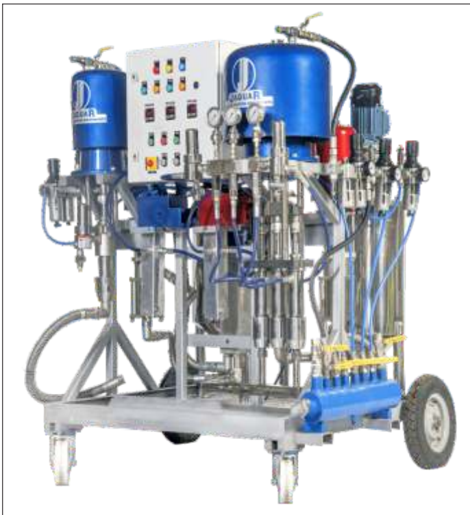
The plural component hot airless spray machine.
