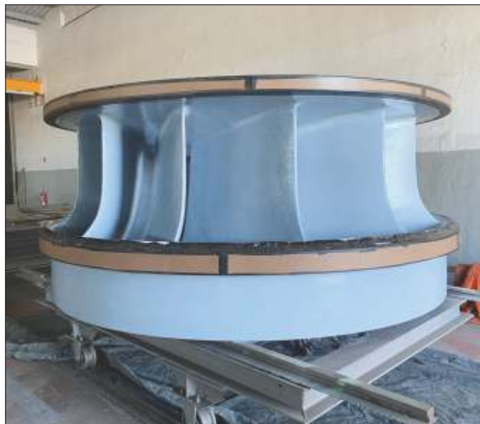
First coat of epoxy coating, Belzona 1341 (Supermetalglide), applied.
