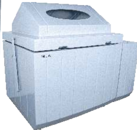
Salt Spray Chamber FRP
