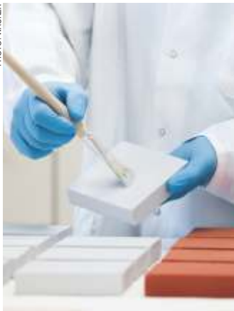
SILRES® BS 338 is a new silicone additive for interior silicate paints and plasters. Coatings modified with this additive are water-repellent, breathable and easy to apply.
