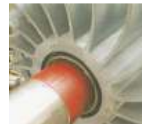
Motor Shaft Coated with Aluma Coat - BR
