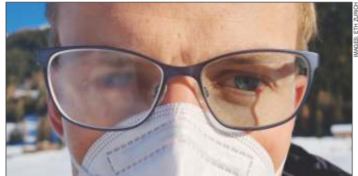
Close-up of man's face. His left lens has the new anti-fogging nanocoating. The other lens is uncoated.
