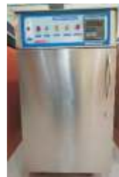
HUMIDITY TESTER ASTM D 2247, ISO 6270
