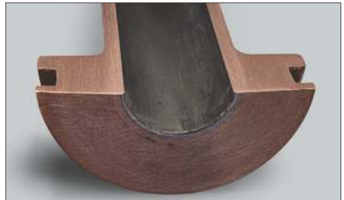
Cross section of a Hardide ® coated copper nozzle after 22 hrs+ service with Stellite 6 Powder showing no pickup present.
