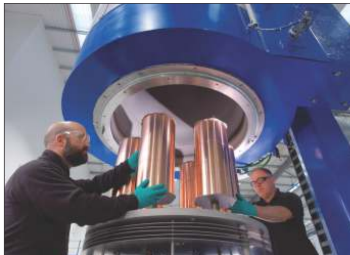
Loading a Hardide® coating reactor.
