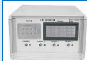
CATHODIC DISBONDMENT TESTER ASTM G 8, G 42, 95 & ISO 15711
