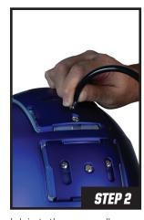
Lubricate the pump needle generously and insert needle as shown. Do not force the needle into the port; doing so may puncture the liner's opposite wall.
