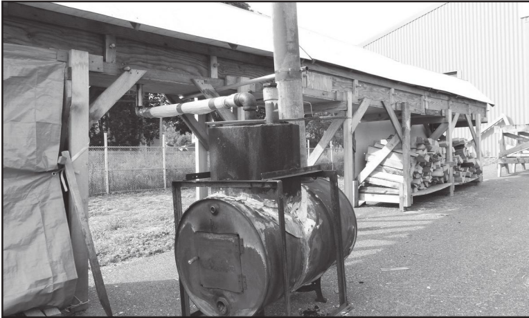
Steambox used to soften and bend stringers and planks. 2014
