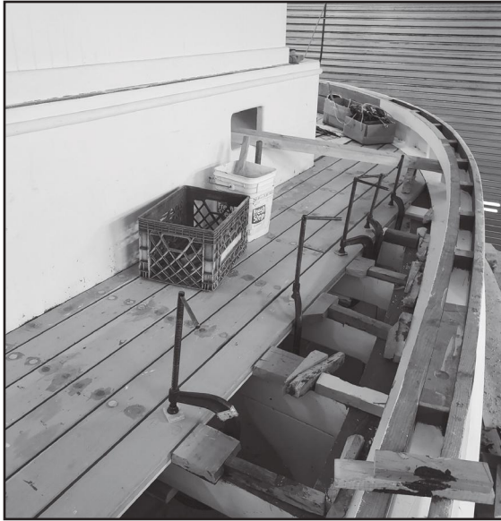
Left: Planking the deck, 2021
