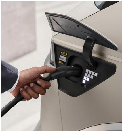
Ultra-fast 800V (350 kW) charging system
