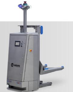
The Palletmover Stainless Steel is a robust, high-performance automated guided vehicle designed for harsh environments. Engineered with durability in mind, its stainless steel construction ensures resistance to corrosion, making it ideal for industries such as food processing or pharmaceuticals.
