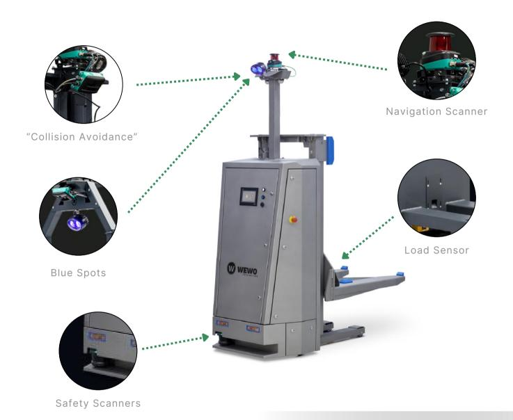
The AGVs are equipped with advanced safety systems designed to protect employees, infrastructure, and the robots themselves.
