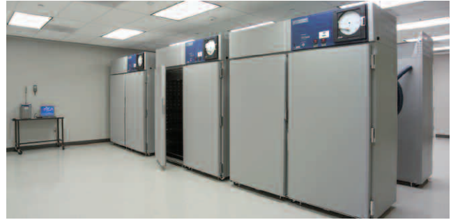
Reach-in environmental chambers
