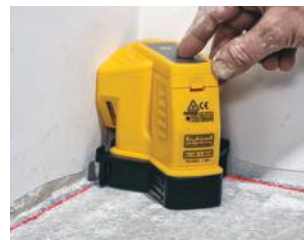
Positions inside corners to check for square
