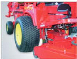
Tires especially for use on grassy surfaces ensure low pressure on the ground
