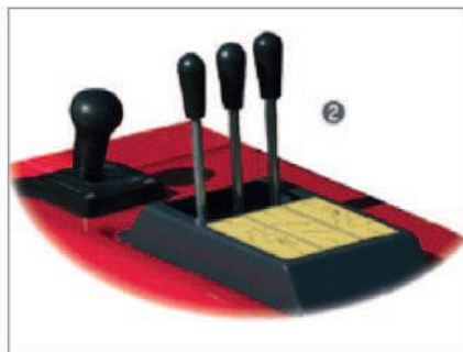
Controls for attachments at the front and rear
