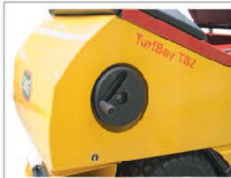
Hand wheel for dedusting of the permanent filter
