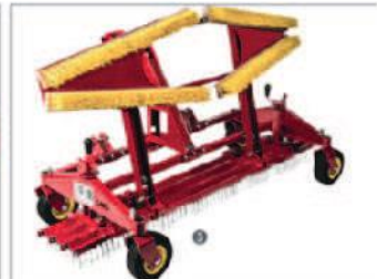
Trailing drag brush, can be folded
