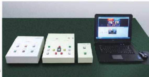
From left, Budo Time Operation Board, Game Operation Board, Time Operation Board, and Team Name/Score Input Device
