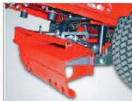
Practical coupling system for mounting all attachments without tools
