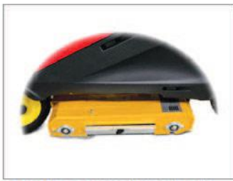
Ground driven rotary brush with adjustable vibrating screen from 4-10 mm
