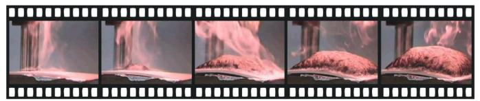
Swelling of a material to a multiple of its original size due to exposure to an external heat source is called intumescence. During the process of swelling the volume of the material increases whereas its density decreases. In an intumescent system a barrier is formed at the sample surface that protects the underlying material thermally from the external heat source and prevents flammable decomposition gases to migrate to the surface.
