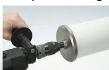
Driven off an adaptor in a power tool, the Soil Pipe Chamfering Tool is designed to remove the burr from around soil pipes to prevent seals being pushed out of fittings when assembled. The carbide grit section chamfers your pipe in seconds and also provides excellent tool durability
