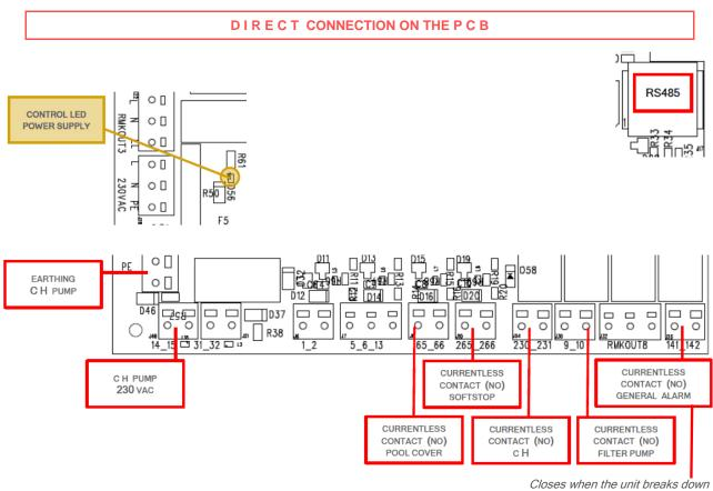
Can be applied in a domotic system to indicate a failure
