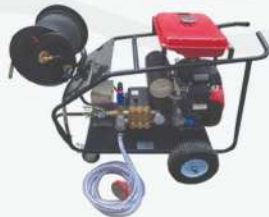
Sewer Pipe Cleaning Machine
