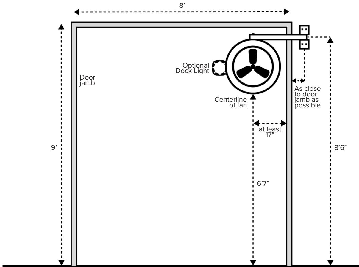
**Note:** The TC-18 is designed to purge a trailer of hot air. Mounting in the top corner pushes air through the trailer and out the opposite corner of the door, as shown below, with an exit velocity of approximately 200 FPM. The fan will not be as effective if positioned other than what is recommended or by directing on an individual.
