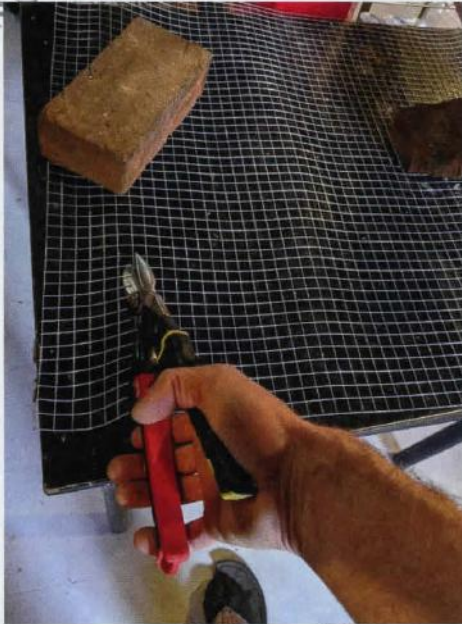
Snip the hardware cloth along the row.
