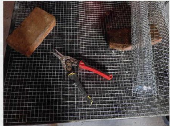
This is all you need to make a simple and inexpensive mouse guard. The hardware cloth is readily available at hardware stores. You'll want 1/2". The bricks are there simply to keep the wire from rolling back on itself.
