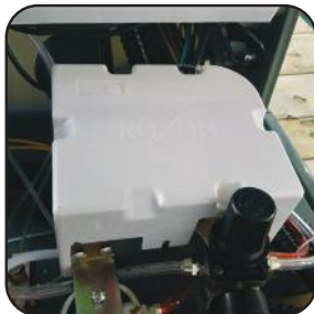
Power protection cover for safety
