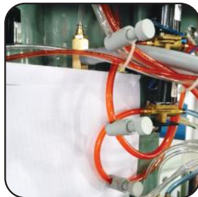
3* regulators for controlling the water flow of cup filling. Spittoon rinsing and air flow of air suction
