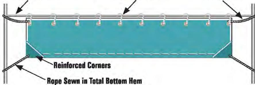
Both variations can be repeated for the bottom of the banner, if required. If the bottom is not secured with a wire guide, we recommend sewing 1/4" poly rope through the bottom hem with extra rope to reach the supporting side structure (see diagram). Reinforcing both bottom corners is recommended.
