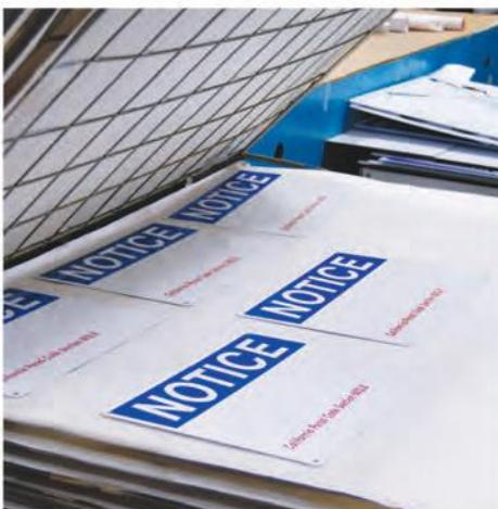
after ink is applied to .080 aluminum with rounded corners and holes
