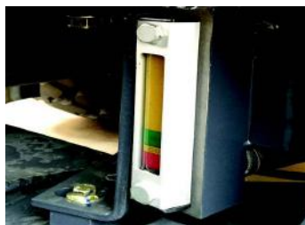
Autolube is a standard feature on the Taylor T-1035. All pressure taps and site gauges are easily accessible. Fluid drains provide environmentally friendly drainage capability and are grouped together for convenient serviceability.
