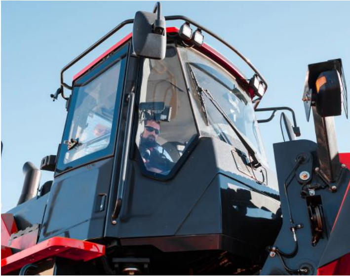
The Taylor T-1035 has been designed to offer optimized visibility. A panoramic view cab with curved front glass has been paired with well-positioned lift arms to allow the operator a clear line of sight to the attachment at ground level.
