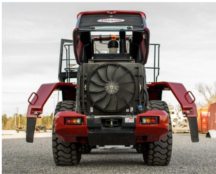
The rear full fenders swing out for easy access to the engine compartment. The electrically actuated, wide opening fiberglass hood of the Taylor T-1035 gives you easy access to the engine and its easy-to-reach service points. The radiator also swings out for ease of service.
