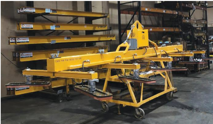
The 7,000-lb. capacity powered vacuum lifter from Caldwell handles laser cut plate steel and has 10 rectangle pads instead of the round pads on standard models.
