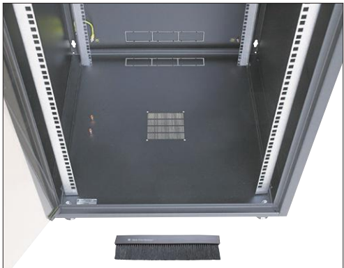
View of the bottom plate in the SJB cabinet. On the back of the cabinet there are cable openings covered with knock-out blanking plate which can be replaced with a brush strip (one brush strip is factory-mounted on the top plate, the other one can be ordered as supplementary accessories).
