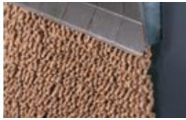
Creation of compressed packaging material with a closed compression flap (HSM ProfiPack P425).
