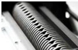
Specially hardened cutting rollers for precision cutting.
