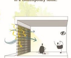
"Use of lattice openings to control sunlight, ensure privacy, and facilitate natural ventilation—reflecting the city's cultural and architectural identity."
