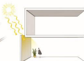
guiding natural light into the interior through skylights offers a contemporary interpretation of light as a life-giving element in Iranian architecture, providing controlled daylight, reducing reliance on artificial lighting, and enhancing ventilation and thermal comfort in Yazd's hot and arid climate
