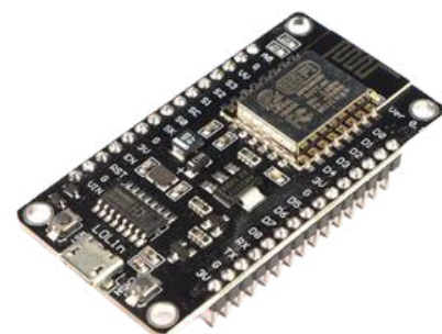
VM 779 NodeMcu ESP8266 CH340 Wifi Development Board
