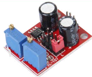
VM 694 NE555 Pulse Frequency Duty Cycle Adjustable Module
