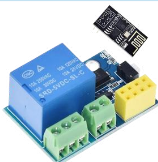
VM 766 ESP8266 WiFi 5V 1 Channel Relay Module
