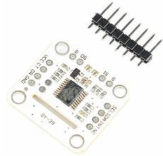
VM 686 TEA5767 Stereo FM Radio Module with Detachable Antenna
