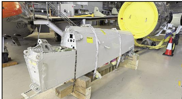
The newly refurbished engine pylon.
