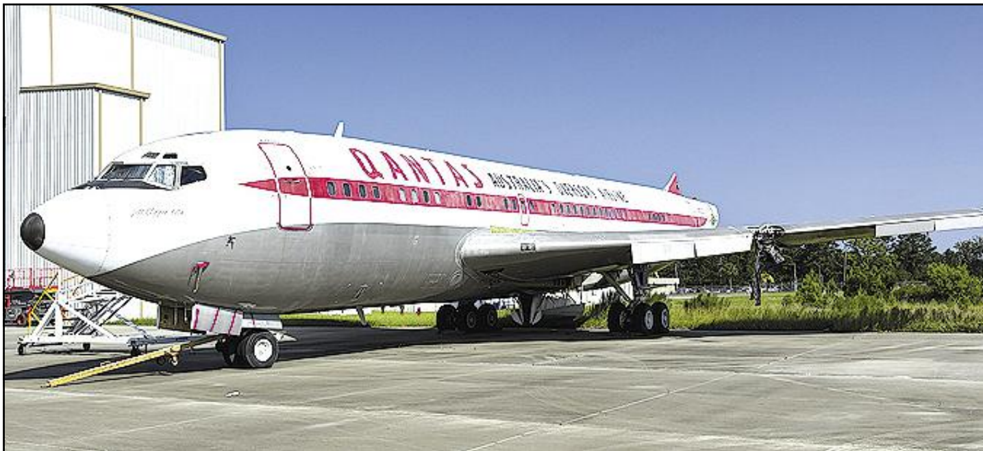
N707JT with engines, flaps and empennage removed.
