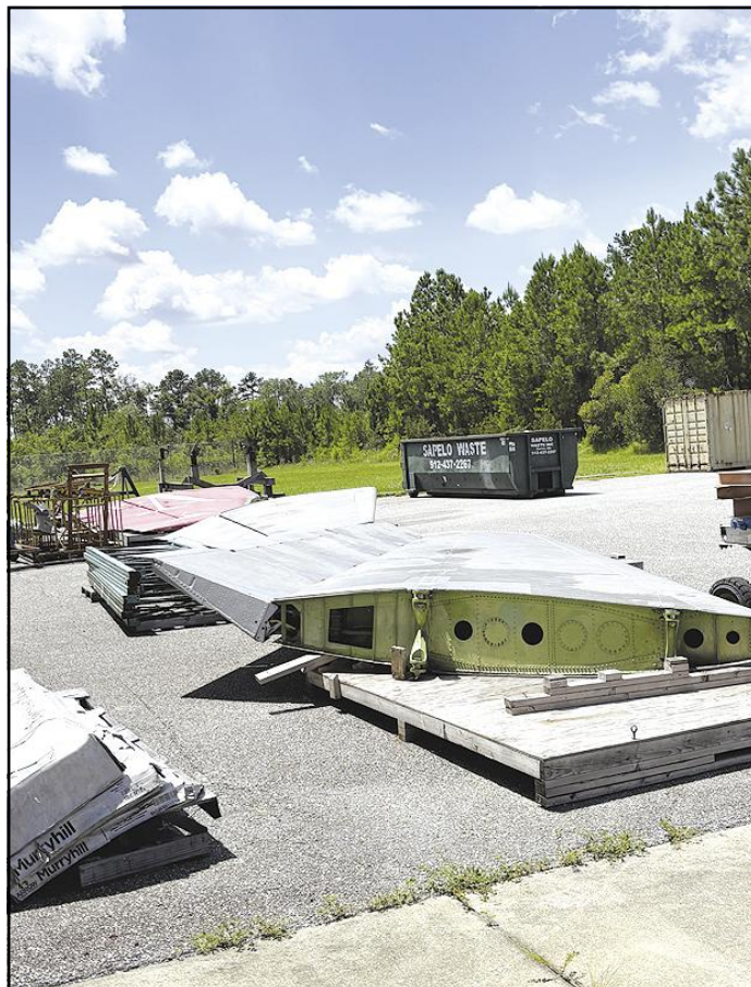
Stabilisers and fin on the ground prior to being lifted.
