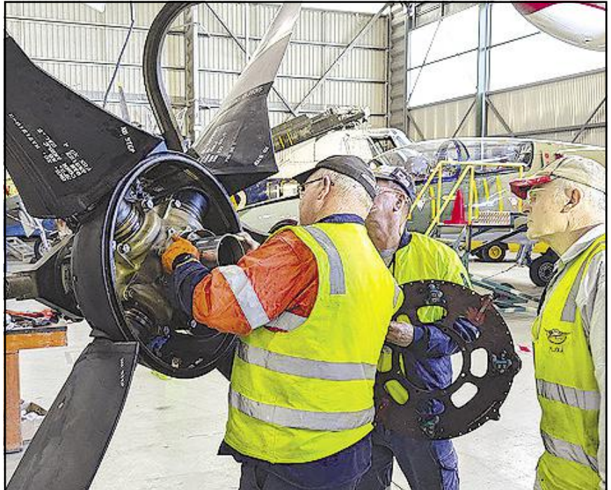
Inspecting the Propeller Hub.
