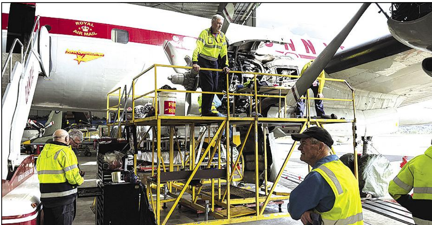
Inspection of the number two engine on Connie.
