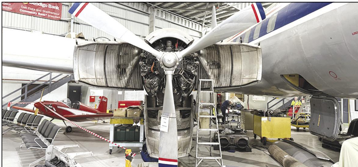
Number 2 engine cowls opened for inspection.
