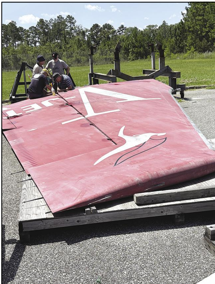
Examining the fin to determine how to remove the rudder.
