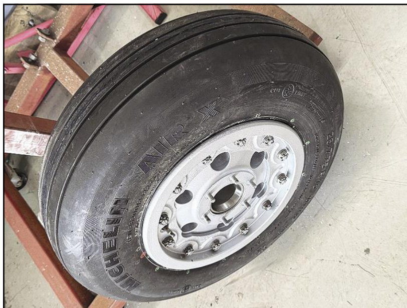
Refurbishing MLG Wheel with new tyre.
