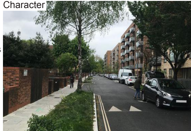
Planting tree pits between car parking spaces.
