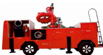
World's First UL Listed 10500 US GPM Foam Monitors For Large Hydro Carbon Tanks
