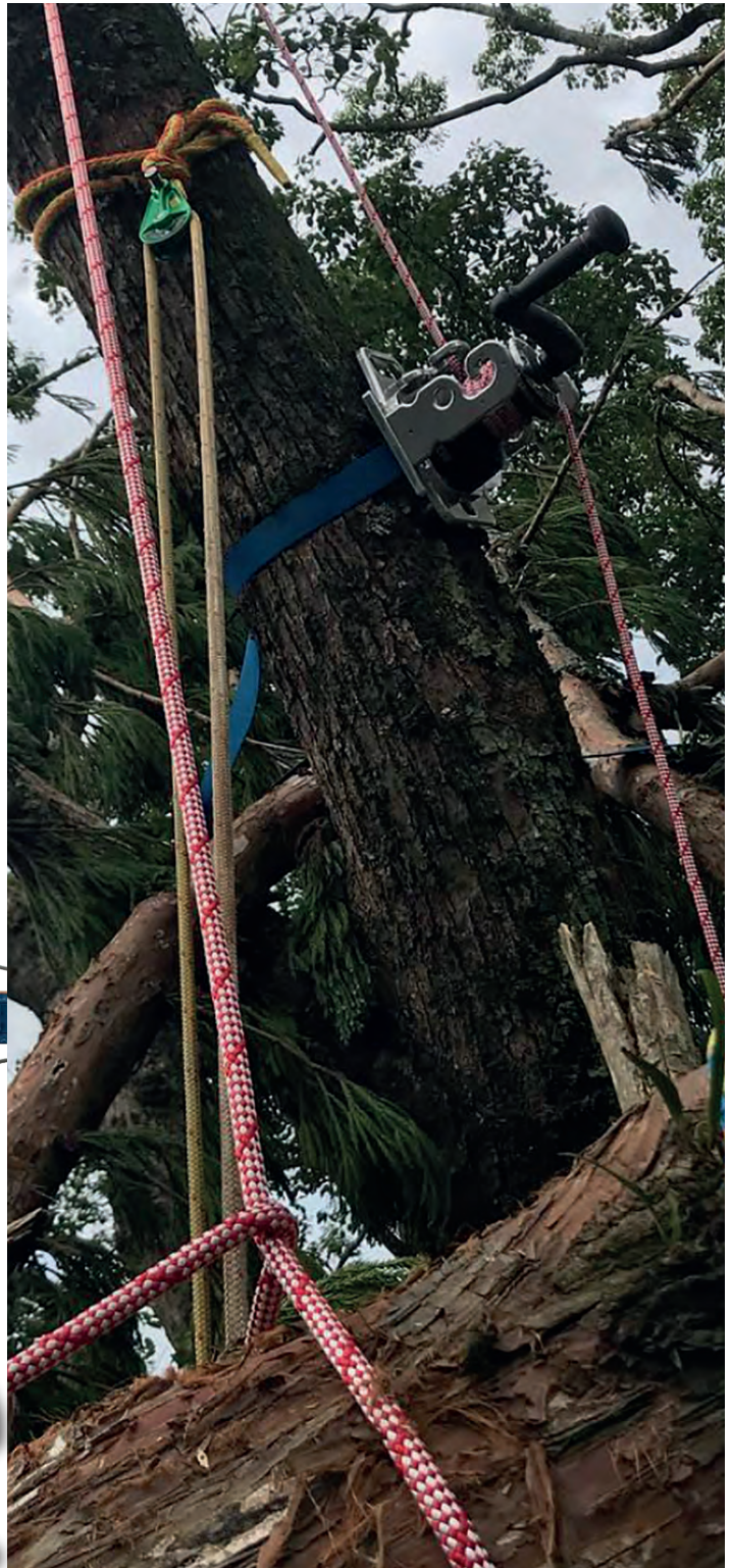
A classic example of where raising is necessary prior to lowering. This is ODSK's Elephant winch from Japan using the ubiquitous Harken capstan and an alloy frame with a trio of unique, machined rope guides which double as friction posts. In this picture the winch is secured to a standing tree used as the anchor from which to raise a faller that is entangled in its branches. This is storm damage from a busy year of typhoons in 2018 and you have little say on where the tree ends up. On another day (with that impact block above the winch), this could have been a congested work area in which a cut section has to be 'unpicked' from an adjacent tree and raised, using the winch, before it can be lowered. It may be an optical illusion but doesn't it look like the ratchet strap on the winch is squeezing the life out of that trunk?
