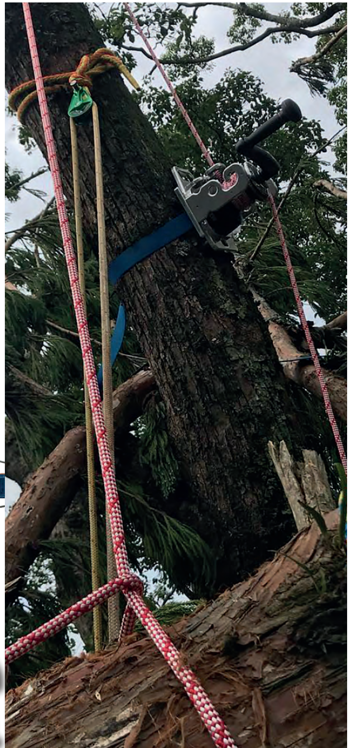
A classic example of where raising is necessary prior to lowering. This is ODSK's Elephant winch from Japan using the ubiquitous Harken capstan and an alloy frame with a trio of unique, machined rope guides which double as friction posts. In this picture the winch is secured to a standing tree used as the anchor from which to raise a feller that is entangled in its branches. This is storm damage from a busy year of typhoons in 2018 and you have little say on where the tree ends up. On another day (with that impact block above the winch), this could have been a congested work area in which a cut section has to be 'unpicked' from an adjacent tree and raised, using the winch, before it can be lowered. It may be an optical illusion but doesn't it look like the ratchet strap on the winch is squeezing the life out of that trunk?
