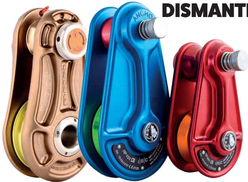
ABOVE Left to right- approximately to scale: DMM Large Impact Block, ISC 3/4" medium and 5/8" small and DMM XS Impact Block. Top right (NOT to scale) the DMM Small Impact Block. Note the hollow spindle on the DMM which is also seen in the Arbortec and TreeUp models. This is for 3D rigging allowing a rope to pass through and redirect or reposition the pulley in free space away from the trunk or to allow a clear route past an obstruction post-arrest. Interestingly, in the TreeUp models the full screw closure is slightly weaker, or perhaps we should say less-strong than their identical pulley with a sprung half turn closure similar to the blue and red ISC pulleys above. ISC's newest model is shown top-right as the series 200 RP248 - the smallest of 3 sizes in a sleek new design.
