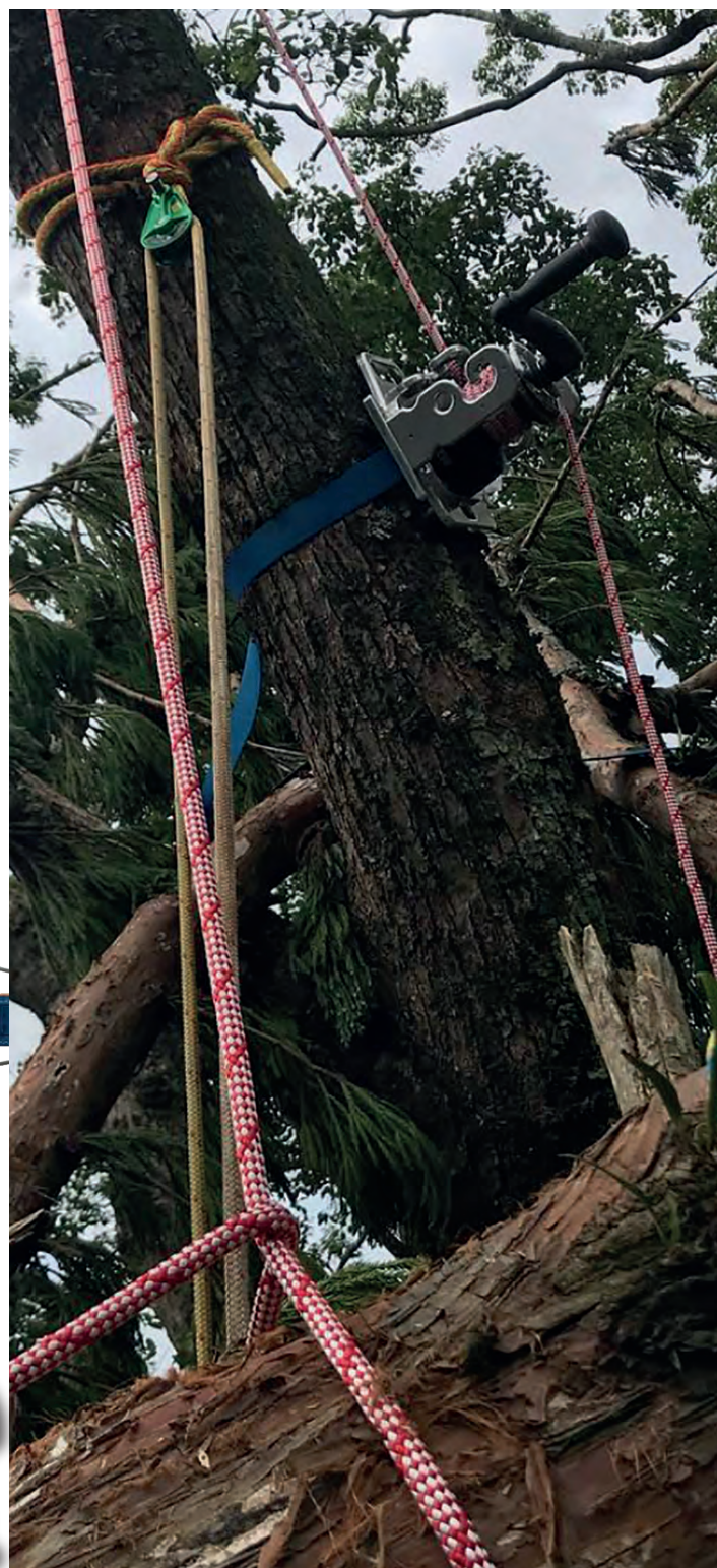
A classic example of where raising is necessary prior to lowering. This is ODSK's Elephant winch from Japan using the ubiquitous Harken capstan and an alloy frame with a trio of unique, machined rope guides which double as friction posts. In this picture the winch is secured to a standing tree used as the anchor from which to raise a faller that is entangled in its branches. This is storm damage from a busy year of typhoons in 2018 and you have little say on where the tree ends up. On another day (with that impact block above the winch), this could have been a congested work area in which a cut section has to be 'unpicked' from an adjacent tree and raised, using the winch, before it can be lowered. It may be an optical illusion but doesn't it look like the ratchet strap on the winch is squeezing the life out of that trunk?
