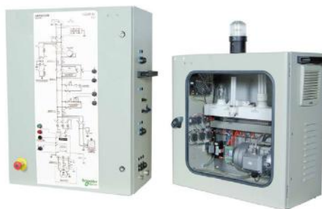
Electrical Network Interference Bench
