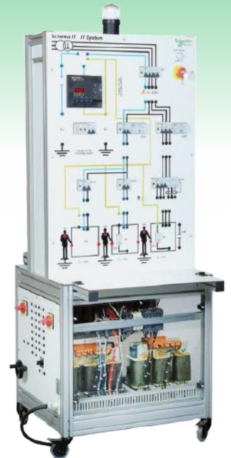
Earthing System Bench
