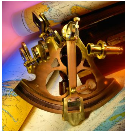
The vertical angle between a celestial body and the horizon can be measured with a sextant. If the vertical angle, the date and the moment of the day are known, the position at sea can be calculated. Photo by Jupiterimages.
