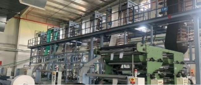
3. Extrusion: mixed formula is then melted, extruded into tubes of film ready for shaping and sealing.
