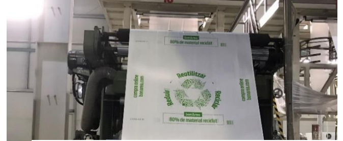
4. Printing: Adjustable automated processes with up to 6 color printing in line.
