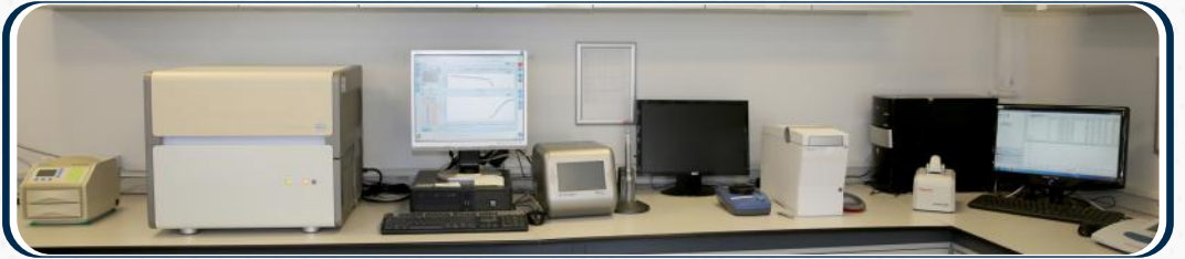
Roche LightCycler 480 II RT-PCR & Invitrogen Neon Por Açma & Agilent Bioanalyzer & Nanodrop 2 UV-Vis
