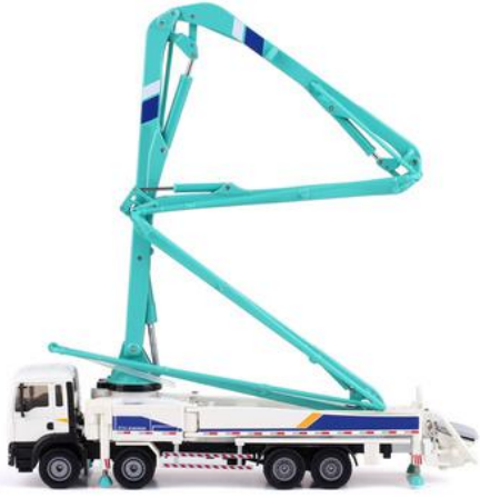
TRUCK-MOUNTED CONCRETE PUMP
