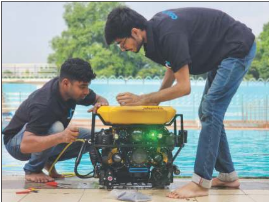
Equipped with high-resolution cameras, ultrasonic thickness gauges, and specialized sensors, the ROVs can inspect submerged surfaces to identify corrosion, metal loss, or marine growth before they become severe.
