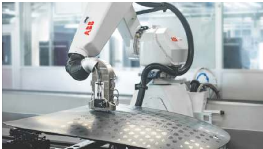
ABB's PixelPaint uses an award-winning paint head similar to an inkjet printer that can apply large areas of color as well as precise details with complete accuracy.
