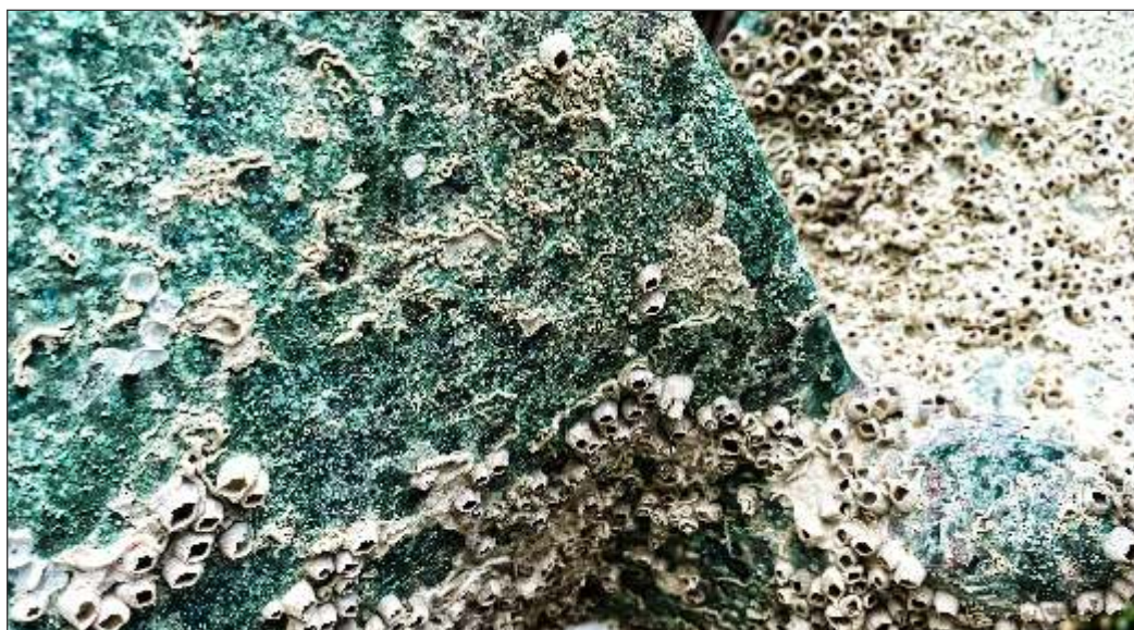
Biofouling – the accumulation of marine organisms on the hull of a ship – reduces the efficiency of the vessel causing it to slow down or to use more fuel to maintain operational speed.
