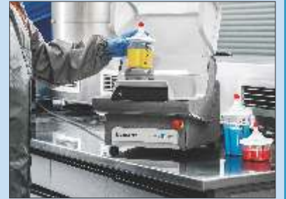
PPG MIX'N'SHAKE™ automated stirring technology replaces manual stirring processes to ensure a homogenized paint mix, complete color accuracy, and a better workplace.
