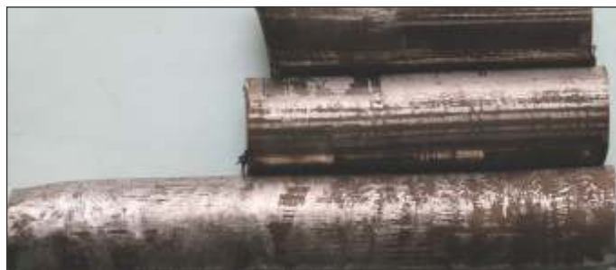
TP316L wet corrosion heat exchanger.
