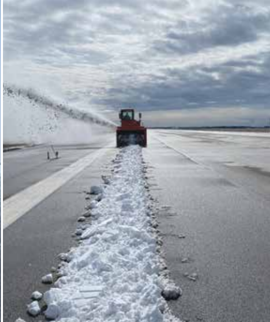
GRF brings with it many new considerations for airport operators. The new rule dictates anything over 25 per cent coverage is equal to 100 per cent coverage and it will certainly change how airports manage their snow removal.
