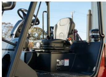
Adjustable Black Vinyl Mechanical Suspension Seat. Adjustable Weight Range to 370 lbs
