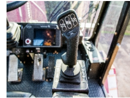
11 Button Command Joystick (Standard)
