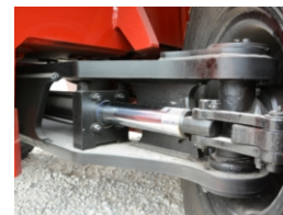
Industry's Toughest Steer Axle (Standard)
