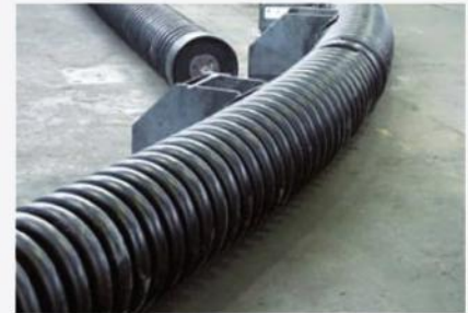
Bending of Durapipes R/D = 30
