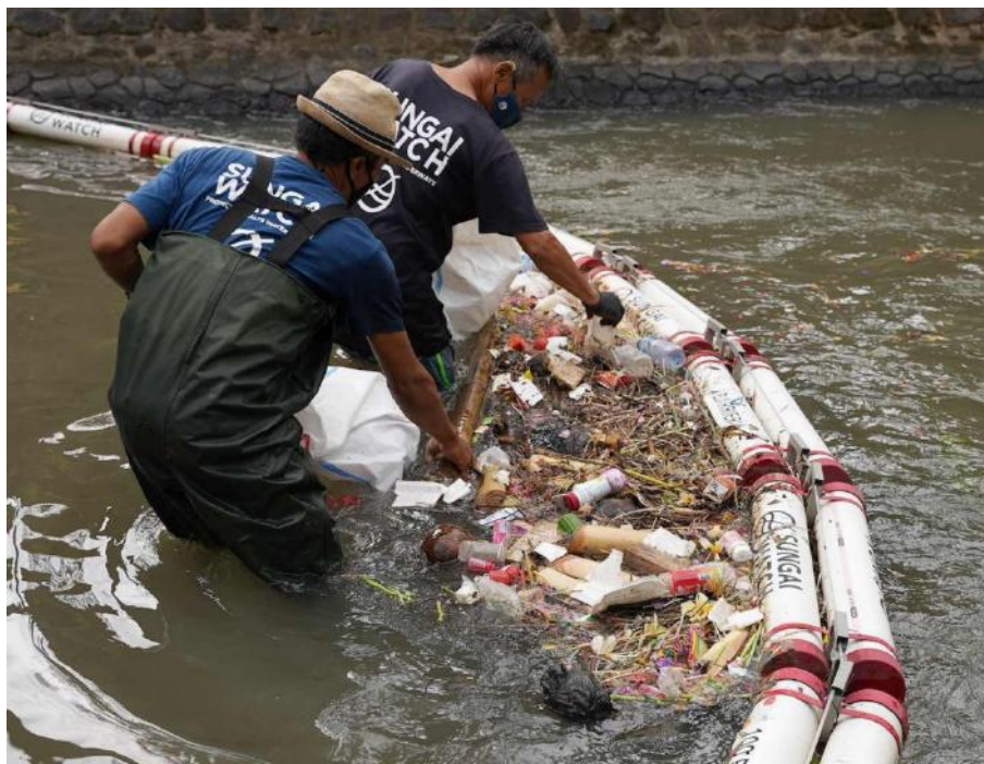
Figure 3. Different types of clean-up technologies across the globe currently work towards cleaning rivers from plastic. Portrayed here is a Barrier employed by Sungai Watch.
