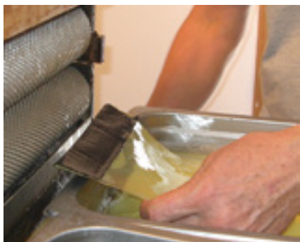
Warm water is used to keep the sheet of beeswax warm as it passes between the cold embossing rollers on the mill. Webster uses a small piece of plastic to protect the forward edge of the wax from getting damaged as it goes through the mill.
