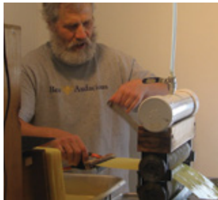
A small hand clamp is used to help ease the sheet of foundation through the mill as the crank is being turned.
