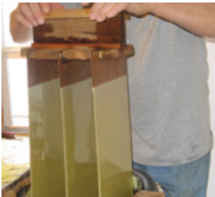
In order to ensure that the sheet of beeswax will not stick to the wood and is easy to remove. The wooden boards are soaked in cold water prior to dipping them into melted beeswax.
