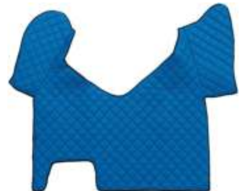
Moqueta A Medida Central Azul Iveco Stralis Automat 02+, Hi-way 12 A 16, Xp 16+ REF: LAM96342
