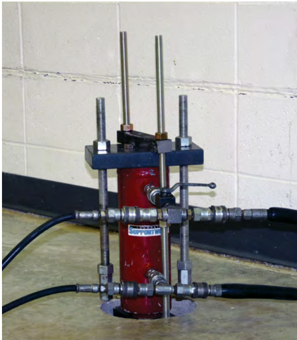
Figure 2.78 Hydraulic connections at lift cylinder
