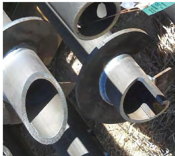
Figure 1.9 45-degree, bevel-cut tip and spiral-cut tip geometry
