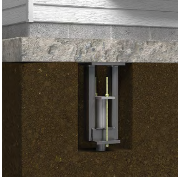
Figure 2.46 Concentric pier installation
