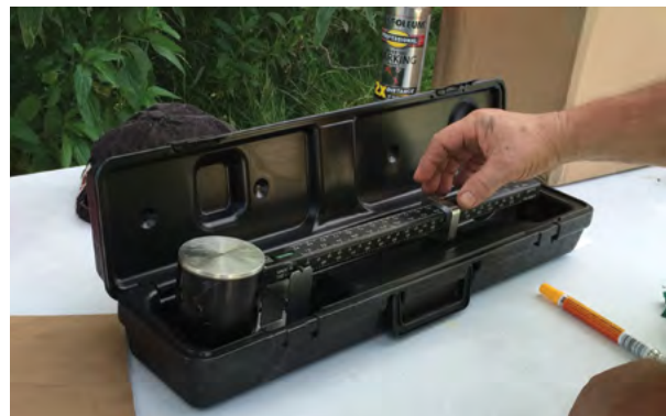
Figure 1.100 Measuring the specific gravity of the grout with a mud balance
