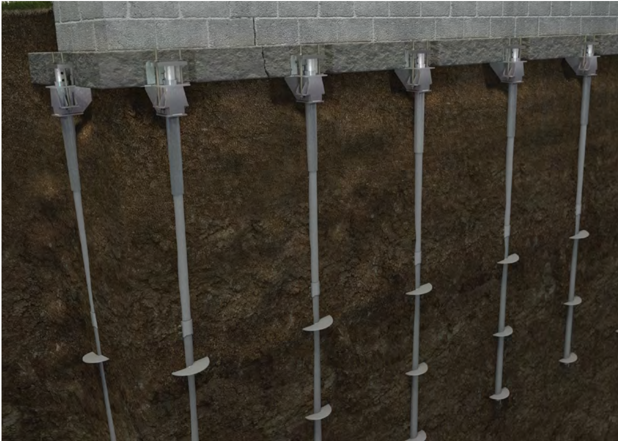
Figure 1.26 Rendering of retrofit helical piers
