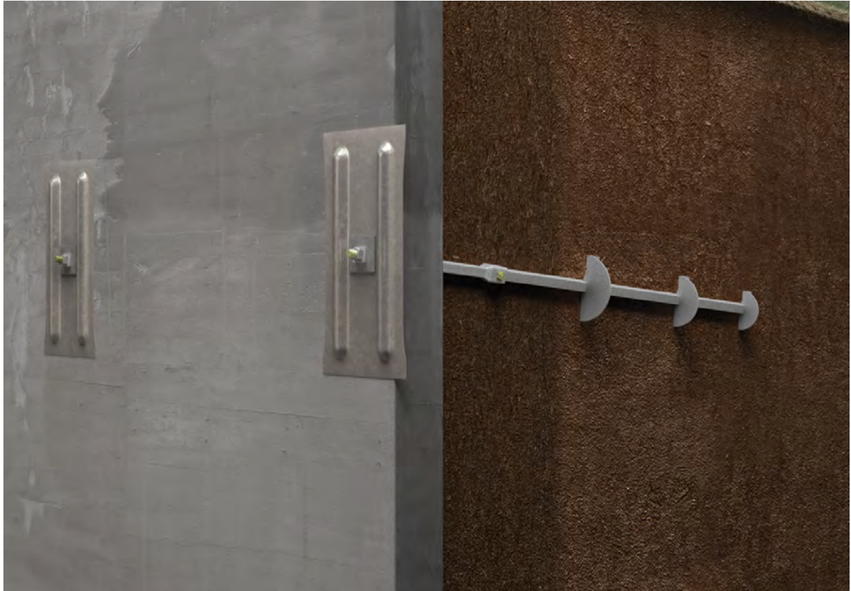
Figure 1.28 Rendering of helical tieback installation
