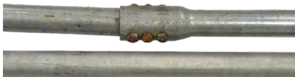
Figure 1.15 Competitor upset coupler variance from straightness
