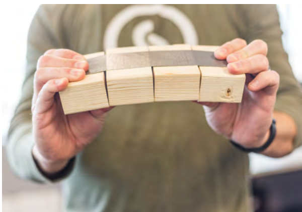
Figure 3.4 CarbonArmor functions similar to a piece of tape on a stack of wooden blocks
