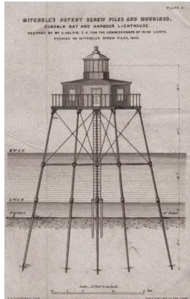
Figure 1.2 Early patent of screw (helical) piles
