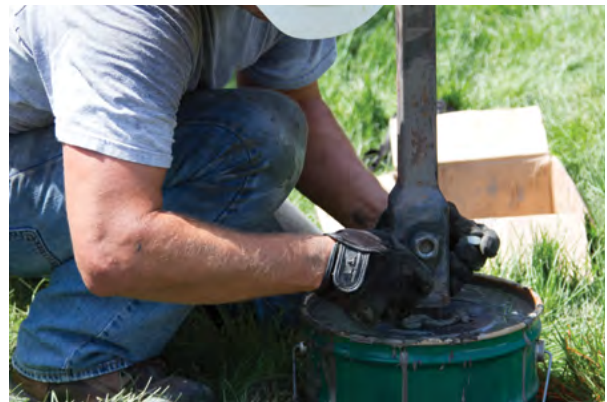
Figure 1.108 Couple the first extension to the lead
