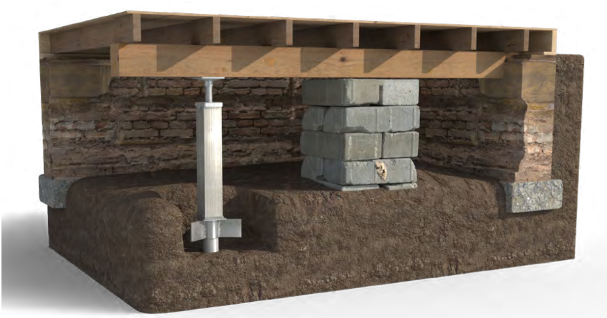
Figure 4.12 Graphic of push pier/SmartJack installation. Backfill around base of SmartJack not shown for clarity. Backfill is required.
