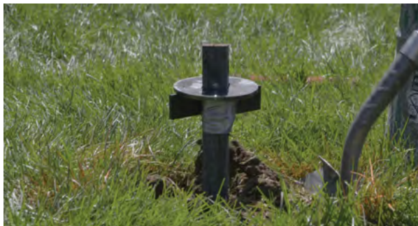
Figure 1.106 Lead displacement plate on the lead section
