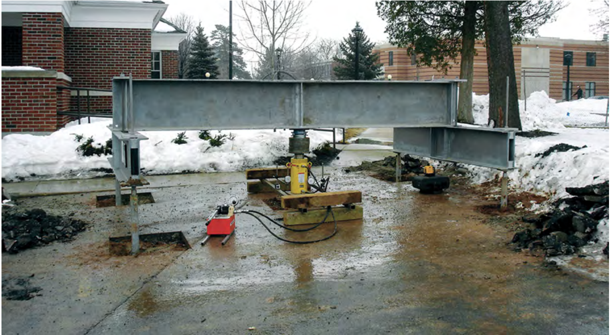
Figure 1.61 Compression load test
