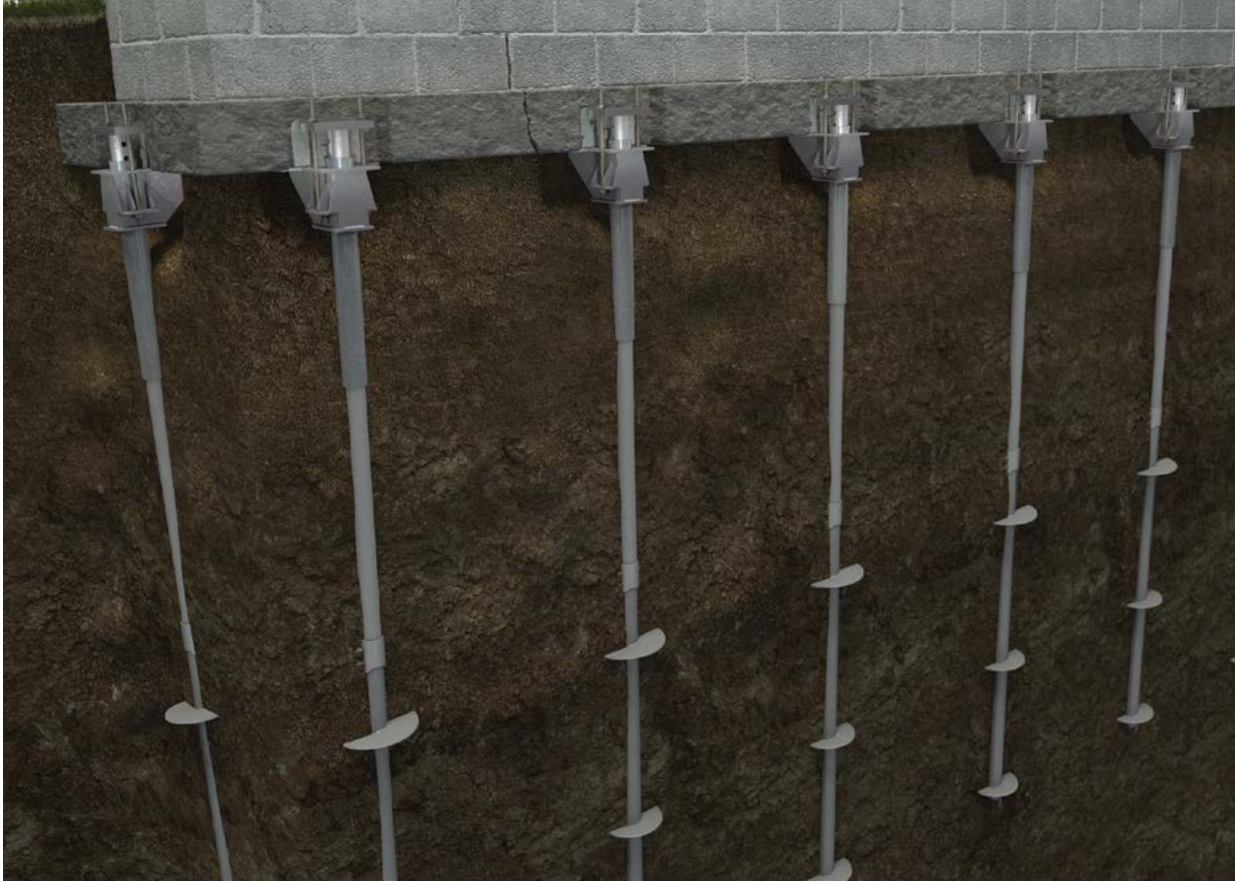
Figure 1.26 Rendering of retrofit helical piers
