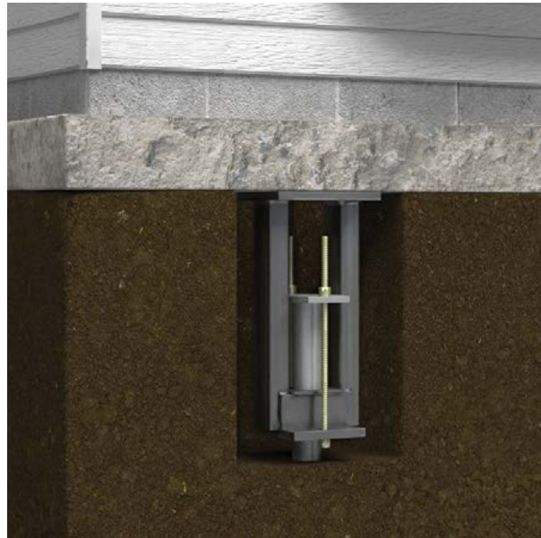
Figure 2.46 Concentric pier installation
