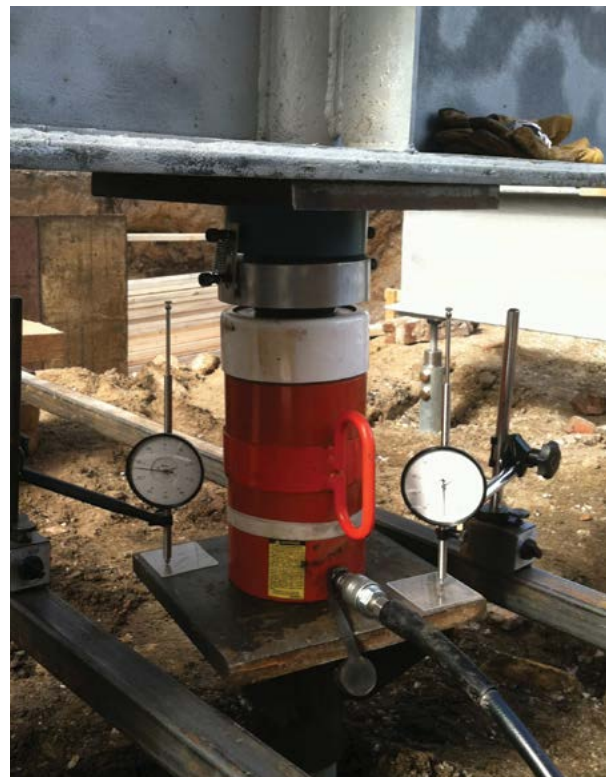
Figure 1.62 Close up of test pile, hydraulic cylinder, dial gauges and hemispherical bearing plate
