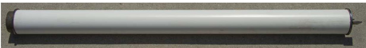
Figure 1.57 PVC casing between lead and first extension displacement plates
