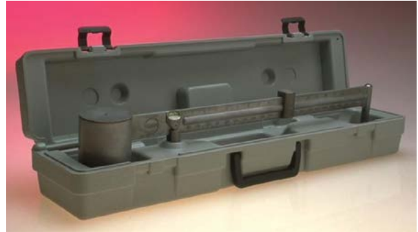
Figure 1.58 Mud balance for specific gravity testing of the grout mixture
