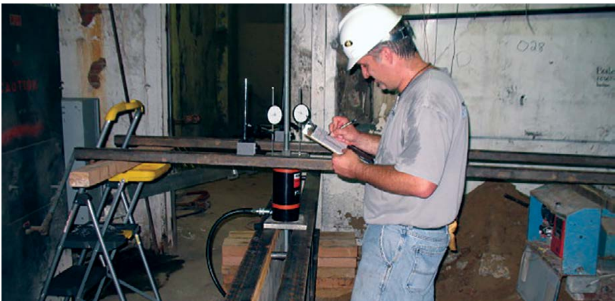
Figure 1.64 Tension load test within basement
