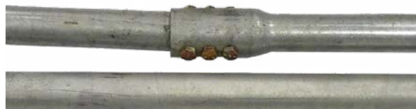
Figure 1.15 Competitor upset coupler variance from straightness
