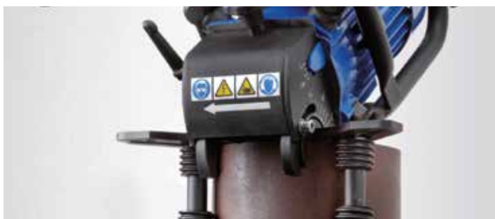
Edge processing of pipes in vertical position.
