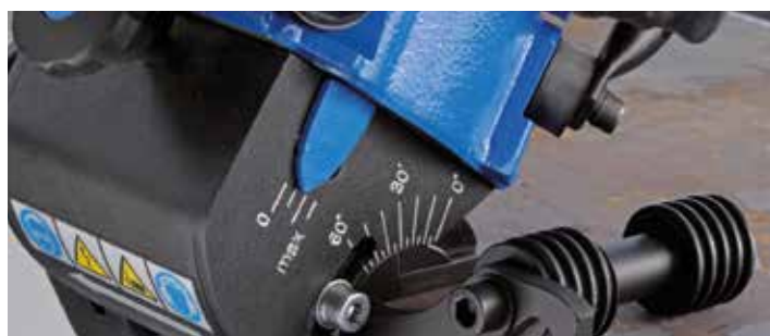
Continuous angle adjustment from 15° to 60°.
