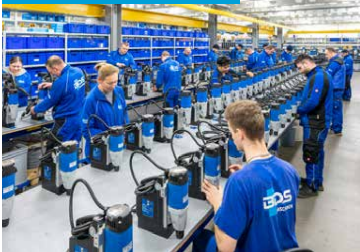
Assembly line for magnetic drilling machines
